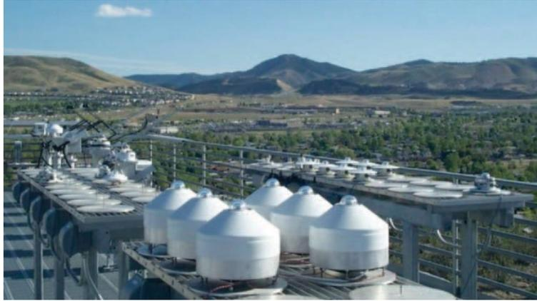
**Figure 3-10. Kipp & Zonen model CM22 pyranometers installed in ventilated CV2 enclosures.**
