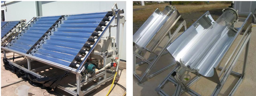
**Figure 8-12. CPC photo-reactors installed at PSA for solar water disinfection applications: (left) CPC-SODIS, (right) FITOSOL-2. (Source: PSA, CIEMAT <http://www.psa.es/en/instalaciones/aguas.php>)**
