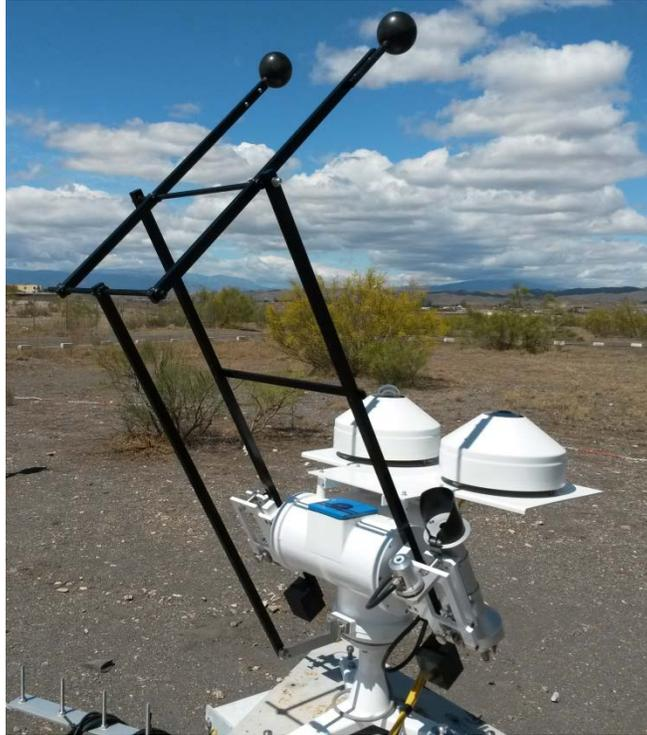
**Figure 3-4. Pyrheliometer, a shaded pyranometer and a shaded pyrgeometer mounted on an automatic solar tracker. Photo from DLR**
